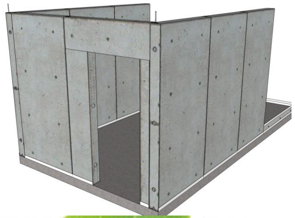
6. Cyclone Tie down rods are installed
