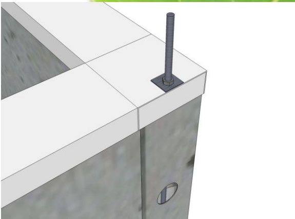
9. Cyclone Rods Are fastened with nut and washer
