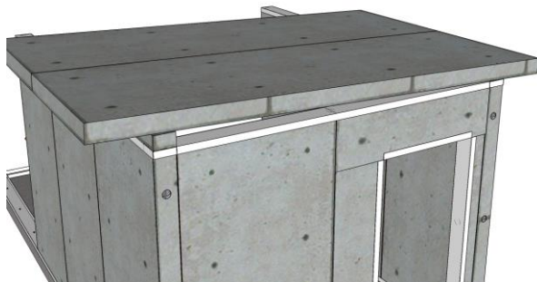
15. Roof Panels are fastened using 170mm TEX Screws
